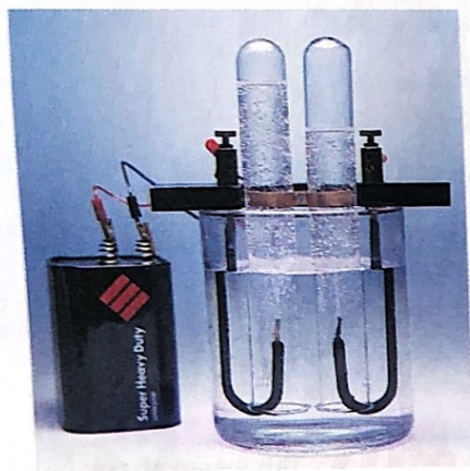
FIGURE 5 When an electric current is passed through water that has been made slightly conductive, the water molecules break down to yield hydrogen (in tube at right) and oxygen (in tube at left). Bubbles of each gas are evidence of the reaction. Note that twice as much hydrogen as oxygen is produced.
