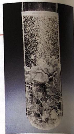
FIGURE 6 Solid zinc reacts with hydrochloric acid to form aqueous zinc chloride and hydrogen gas.
