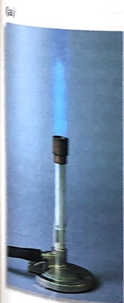
FIGURE 3 (a) In a Bunsen burner, methane combines with oxygen in the air to form carbon dioxide and water vapor. (b) The reaction is represented by both a molecular model and a balanced equation. Each shows that the number of atoms of each element in the reactants equals the number of atoms of each element in the products.
