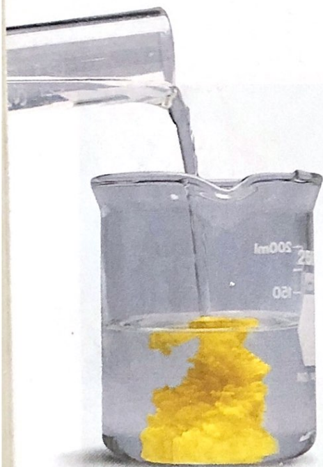
FIGURE 12 The double-displacement reaction between aqueous lead(II) nitrate, \text{Pb}(\text{NO}_3)_2(aq) , and aqueous potassium iodide, \text{KI}(aq) , yields the precipitate lead(II) iodide, \text{PbI}_2(s) .
