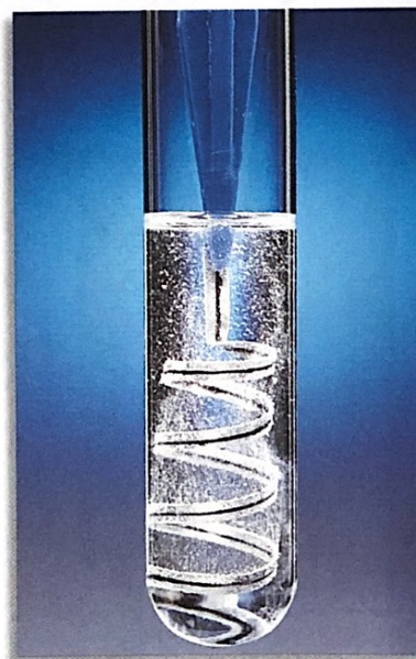
FIGURE 11 In this single-displacement reaction, the hydrogen in hydrochloric acid, \text{HCl} , is replaced by magnesium, \text{Mg} .
